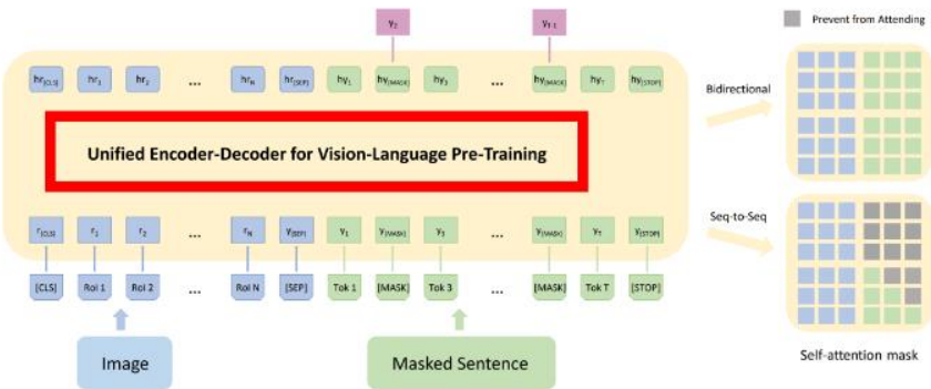
Figure 2: Model architecture for pre-training. The input comprises of image input, sentence input, and three special tokens ([CLS], [SEP], [STOP]). The image is processed as N Region of Interests (RoIs) and region features are extracted according to Eq. 1. The sentence is tokenized and masked with [MASK] tokens for the later masked language modeling task. Our Unified Encoder-Decoder consists of 12 layers of Transformer blocks, each having a masked self-attention layer and feed-forward module, where the self-attention mask controls what input context the prediction conditions on. We implemented two self-attention masks depending on whether the objective is bidirectional or seq2seq. Better viewed in color.
